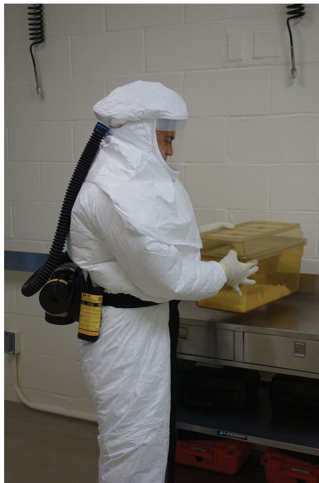
Figure 14-3. Another view of a powered air-purifying respirator. Researchers also use BioSafety Level 4 “blue suits” (not pictured). Auscultation of animals using a stethoscope is also not possible while wearing a “blue suit.” Photo courtesy of the US Army Medical Research Institute of Infectious Diseases, Ft Detrick, Maryland.
