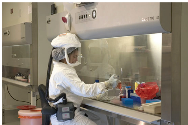
Figure 14-2. Researcher using a powered air-purifying respirator (PAPR). Auscultation of animals using a stethoscope is not possible while wearing a PAPR. Photo courtesy of the US Army Medical Research Institute of Infectious Diseases, Ft Detrick, Maryland.
